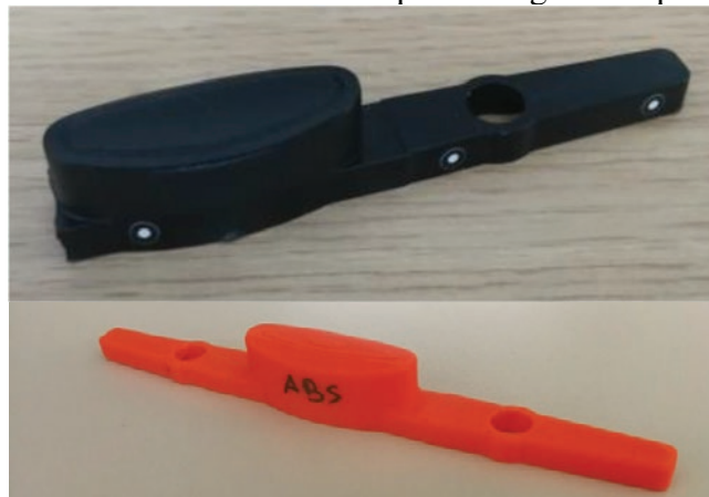
Fig. 1: Top: original part, bottom: final version of redeveloped part
