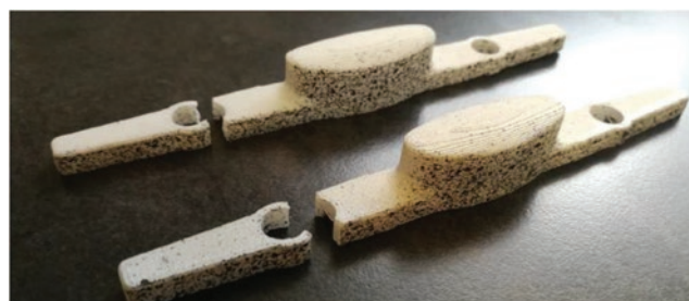
Fig. 12: 3-point overloaded bend test of final part
